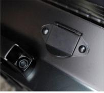
The lock functions as a slam lock, the key is used to unlock the top lid and it locks automatically when the lid is closed. The lock can not stay unlocked.
