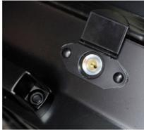
The lock is keyed alike, 2 keys are provided per lock. The key is a standard size and can be duplicated by a locksmith.
